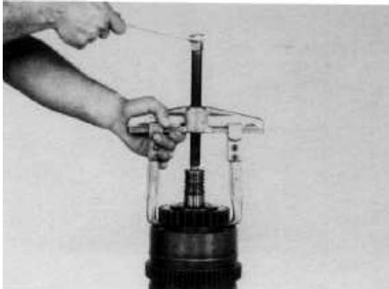
Figure 111 Remove clutch gear and outer bearing.
