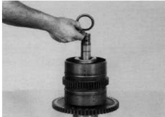
Figure 117 Remove retainer ring retaining washer.
