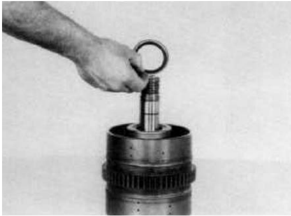
Figure 176 Remove retainer ring retaining ring.
