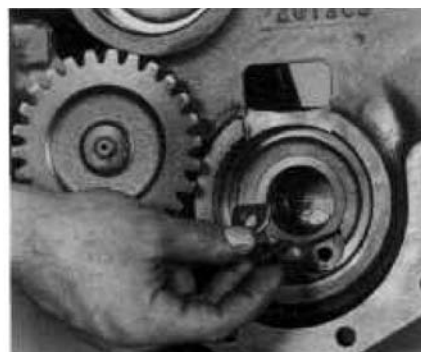
Figure 214 Remove screw and sleeve lock.
