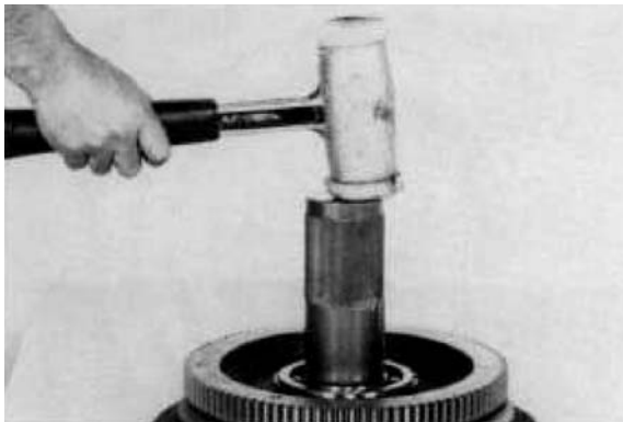
Figure 296 Install impeller cover bearing.
