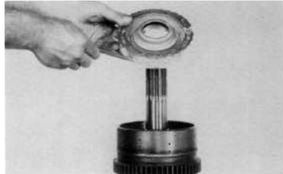
Figure 131 Remove clutch piston.
