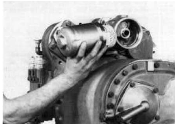
Figure 321 Install new filter element and filter housing.
