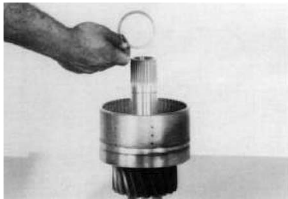
Figure 81 Remove piston return disc spring retainer ring retainer washer.
