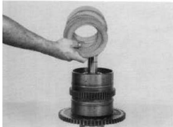
Figure 114 Remove inner and outer clutch discs.
