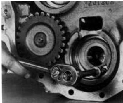
Figure 213 Remove oil sealing ring sleeve retainer screw.
