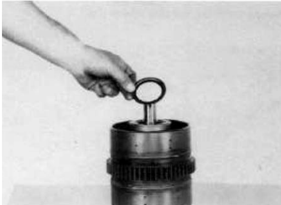
Figure 183 Remove retainer ring retaining washer.
