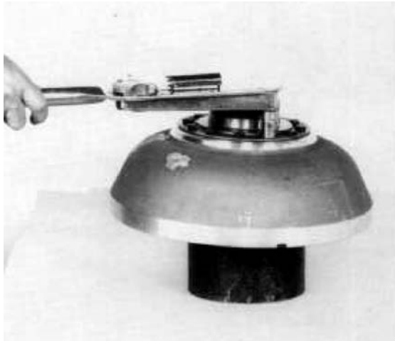
Figure 287 Install (12) impeller hub special screws to approximately .06 inch (1,5) of seated position. With a calibrated torque wrench, tighten screws to 40-45 lbs. ft. [54,3-61.0 N.m.] torque. NOTE: Assembly of impeller to impeller hub must be completed within a fifteen minute period from start of screw installation. The screws are prepared with a coating which begins to harden after installation in the impeller hub holes. If not tightened to proper torque within the fifteen minute period, insufficient screw clamping tension will result. The special screw is to be used for one installation only. If the screw is removed for any reason it must be replaced.
