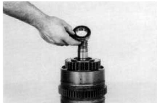
Figure 204 Install clutch gear outer bearing. NOTE: Outer bearing has a shield in it, this shield must be down.
