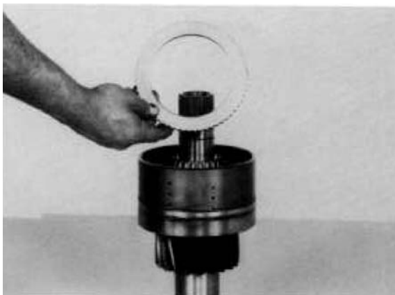
Figure 78 Remove end plate.
