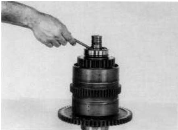
Figure 159 Position end plate lock ball in clutch shaft.
