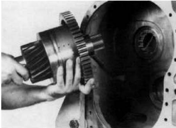
Figure 58 Remove 1st speed clutch assembly.
