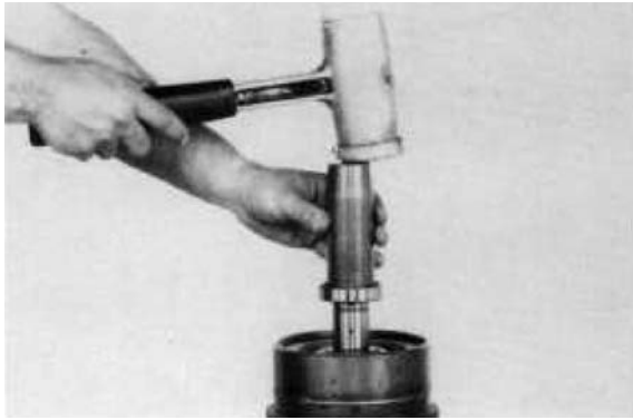
Figure 153 Install clutch gear inner bearing. NOTE: This bearing does not have a shield in it.
