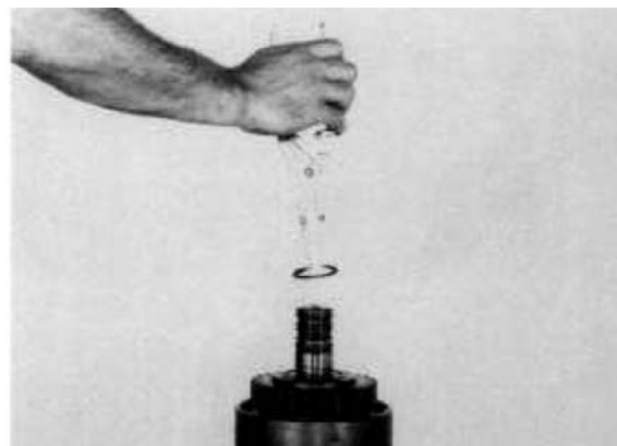
Figure 169 Remove clutch gear outer bearing retainer ring.
