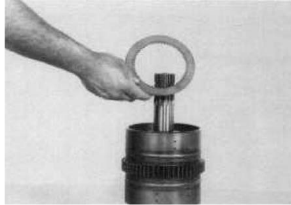
Figure 137 Install one friction disc. Alternate steel and friction discs until the proper amount of discs are installed. First disc next to the piston is steel, last disc installed in friction.
