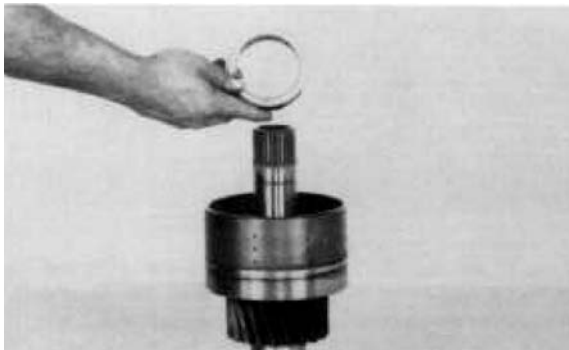
Figure 84 Remove return spring to piston spacer. Turn clutch over and tap clutch shaft on a block of wood to remove clutch piston.
