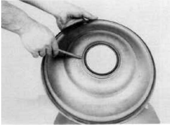
Figure 288 Apply a light coat of Permatex No. 2 on the outer diameter of the oil baffle seal. Press seal in oil baffle with lip of seal down.
