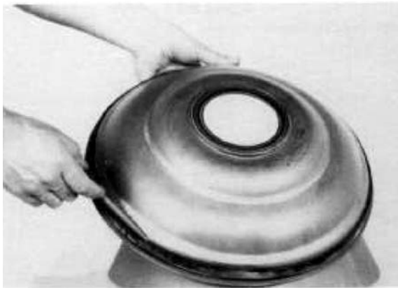
Figure 289 Install new oil baffle seal ring. Position oil baffle on impeller and hub assembly.
