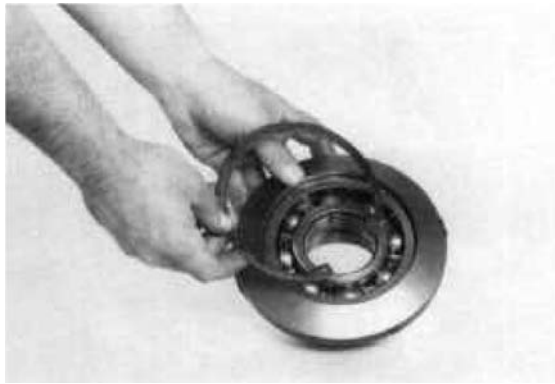
Figure 280 Remove hub bearing retainer ring.
