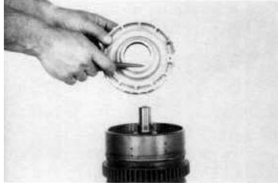
Figure 185 Remove clutch piston.
