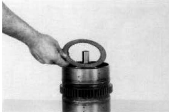
Figure 191 Install one friction disc. Alternate steel and friction discs until the proper amount of discs are installed. First disc next to the piston is steel, last disc installed is friction
