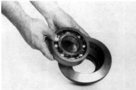
Figure 281 Remove hub bearing.
