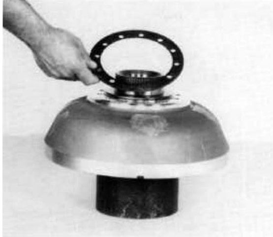
Figure 286 Position backing ring on impeller.
