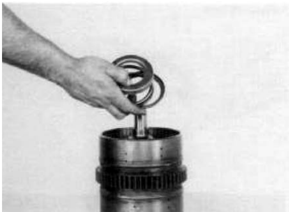
Figure 184 Remove return spring retainers and spring.
