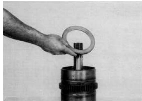
Figure 126 Remove end plate.
