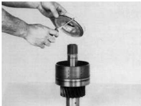
Figure 85 Install clutch piston outer seal ring.
