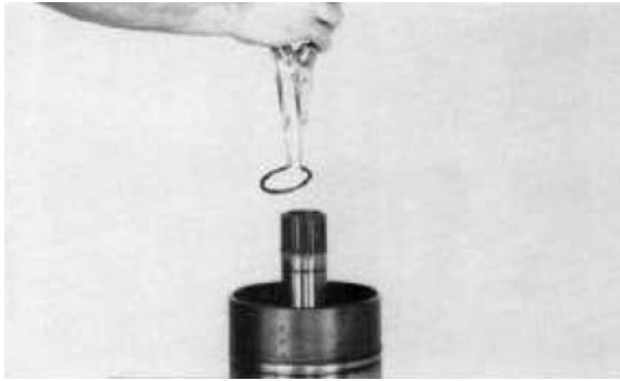
Figure 82 Remove return disc spring retainer ring.
