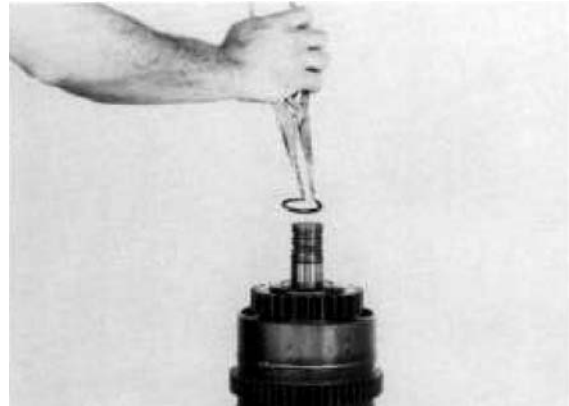
Figure 156 Install clutch gear outer bearing retainer ring.
