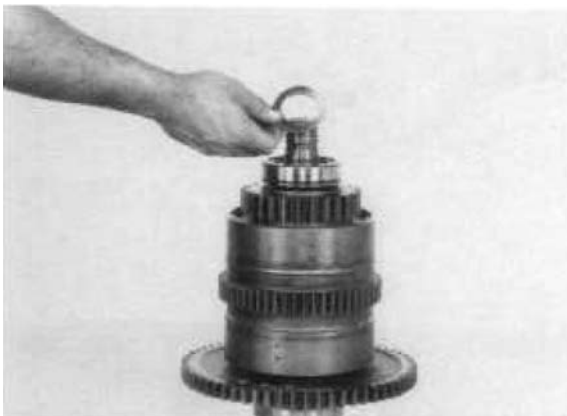
Figure 160 Install bearing end plate, aligning notch in plate with lock ball.
