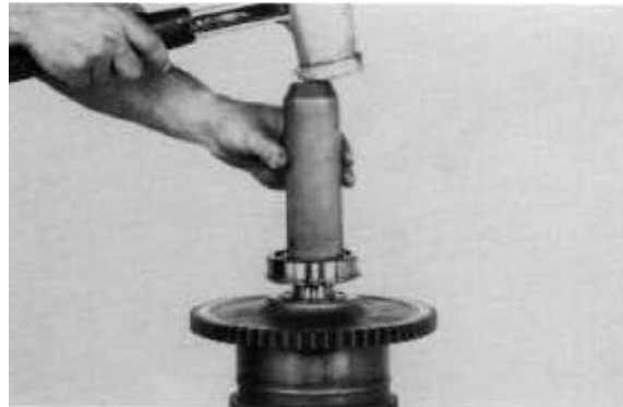
Figure 144 Install 3rd speed clutch shaft rear bearing. NOTE: Bearing outer diameter locating ring must be down.
