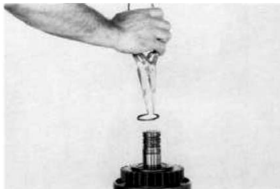
Figure 205 Install bearing retainer ring.
