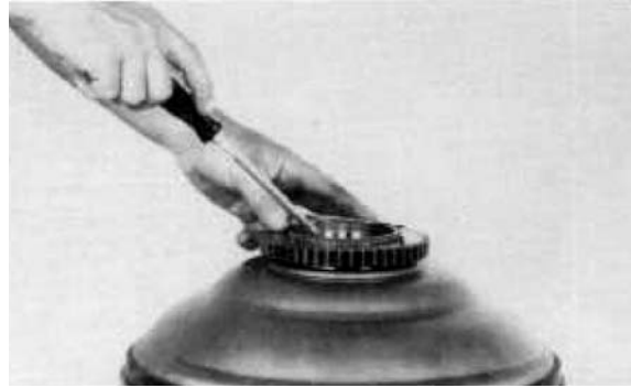
Figure 291 Install pump drive gear retainer ring.
