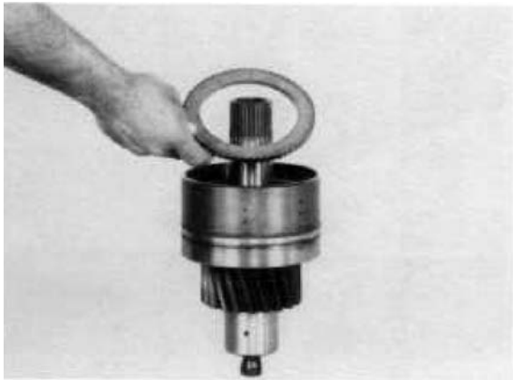
Figure 93 Install clutch disc end plate.
