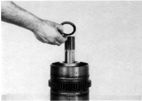
Figure 129 Remove retainer ring retaining washer.
