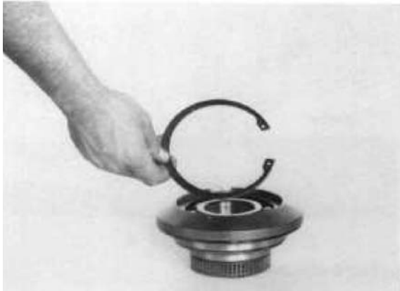
Figure 283 Install bearing retainer ring.
