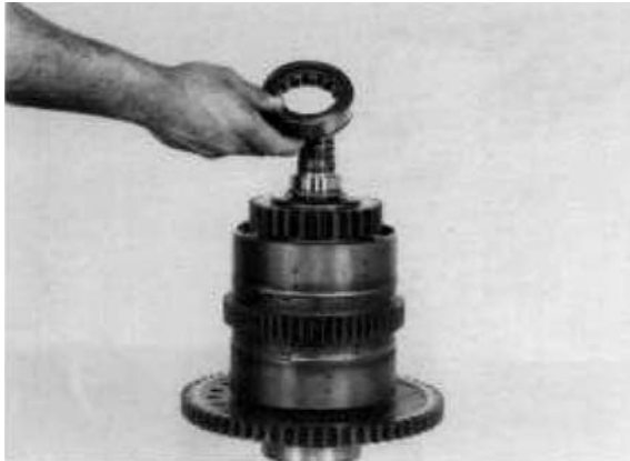
Figure 158 Position front bearing over bearing race.
