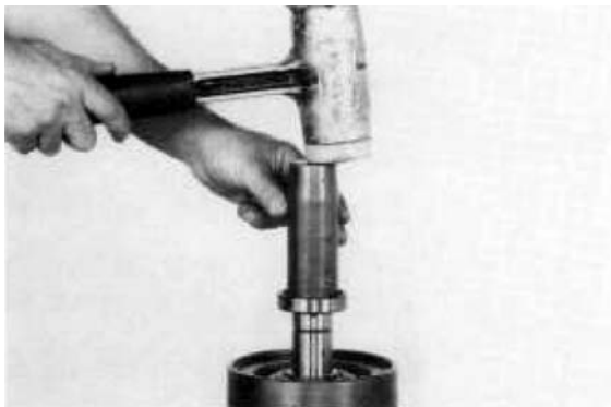
Figure 202 Install clutch gear inner bearing. NOTE: This bearing does not have a shield in it.
