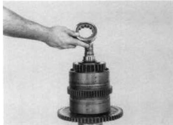
Figure 107 Remove front bearing.
