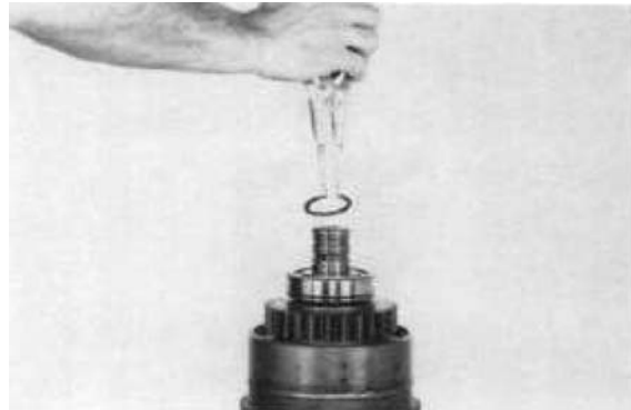
Figure 161 Install bearing retainer ring.
