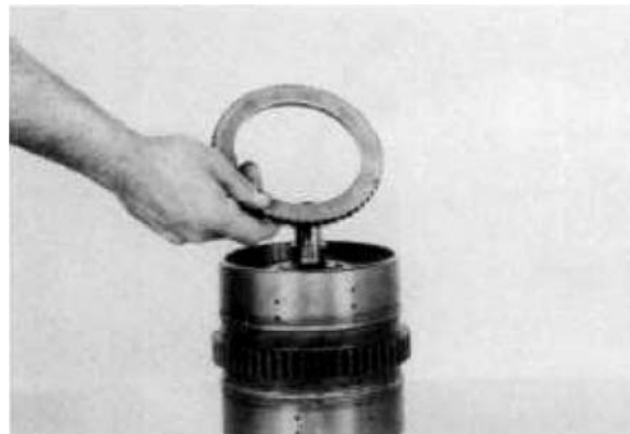
Figure 180 Remove end plate.
