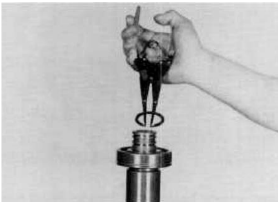
Figure 13 Install bearing retainer ring.
