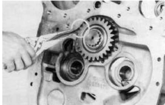
Figure 220 Install drive gear retainer ring.
