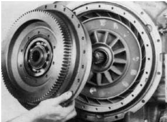
Figure 306 Position turbine and impeller cover on turbine shaft.
