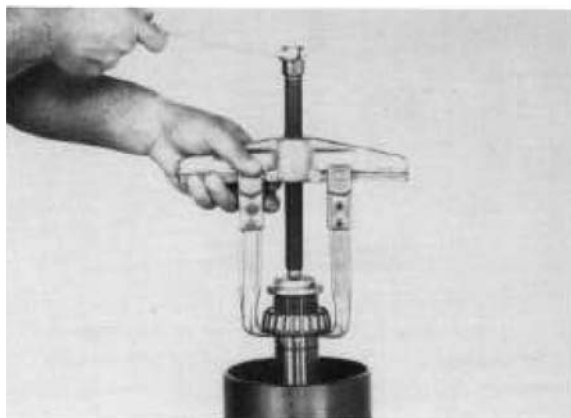
Figure 80 Remove inner taper bearing.
