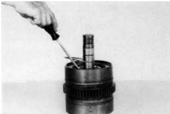
Figure 201 Install end plate retainer ring.
