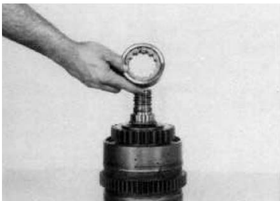
Figure 166 Remove front bearing.
