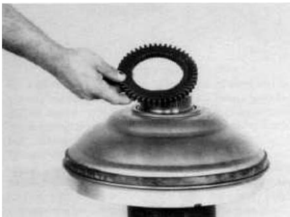
Figure 290 Install pump drive gear on impeller hub.
