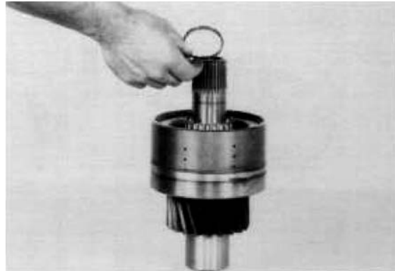
Figure 96 Position taper bearing spacer on shaft.
