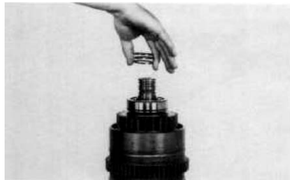
Figure 162 Install clutch shaft piston rings and expander springs as explained on page 79.
