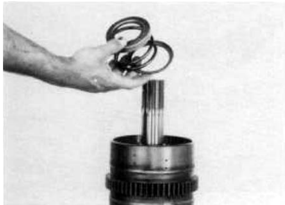
Figure 130 Remove return spring retainers and spring.
