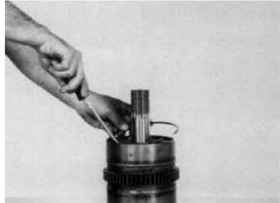
Figure 125 Remove clutch disc end plate retainer ring.
