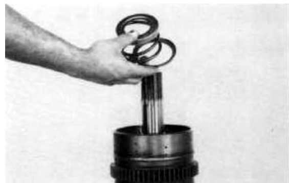
Figure 133 Position the inner return spring retainer, the return spring and the outer spring retainer on clutch shaft.
