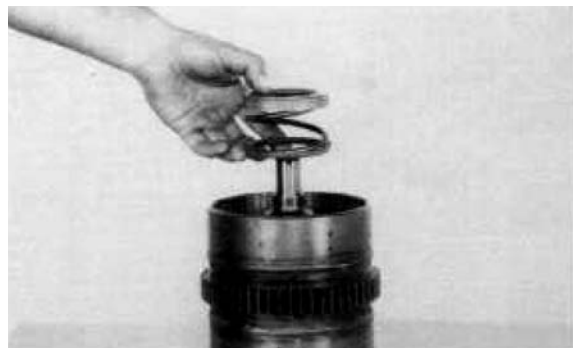
Figure 187 Position the inner return spring retainer, the return spring and outer spring retainer on clutch shaft.
