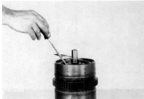
Figure 179 Remove clutch disc end plate retainer ring.
