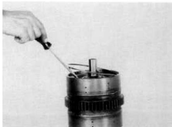
Figure 193 Install end plate retainer ring.
