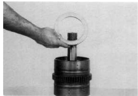
Figure 138 Install clutch disc end plate.
