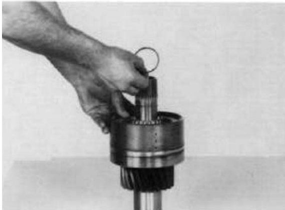
Figure 76 Remove taper bearing spacer.
