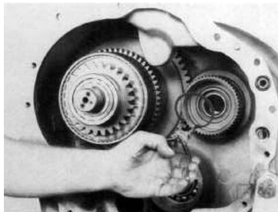
Figure 264 Install disc hub ring retainer retaining ring.
