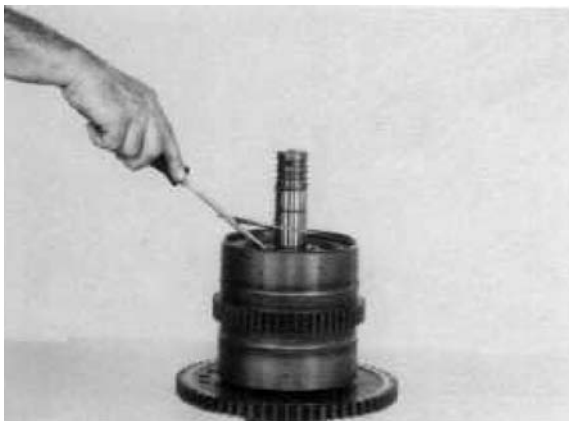
Figure 112 Remove clutch disc end plate retainer ring.
