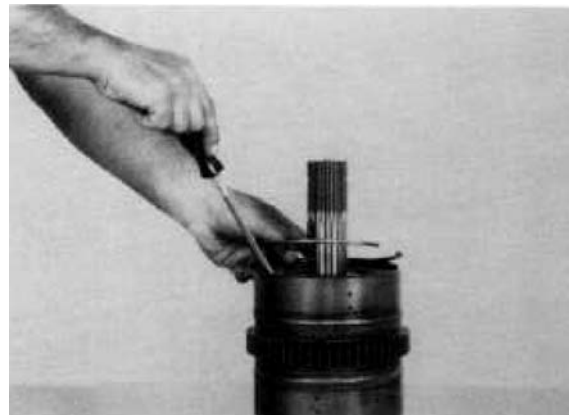
Figure 139 Install end plate retainer ring.
