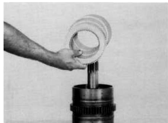
Figure 127 Remove inner and outer clutch discs.
