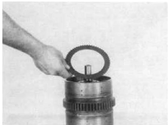
Figure 190 Install one steel disc.
