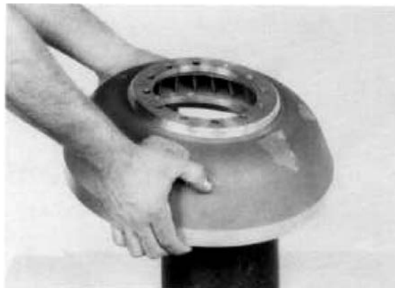
Figure 285 Align holes in impeller with holes in impeller hub.
