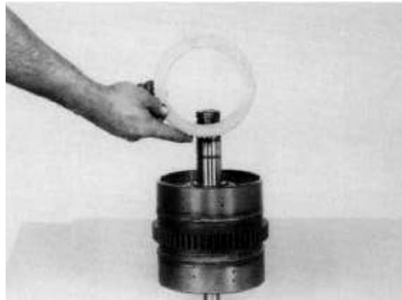
Figure 173 Remove end plate.
