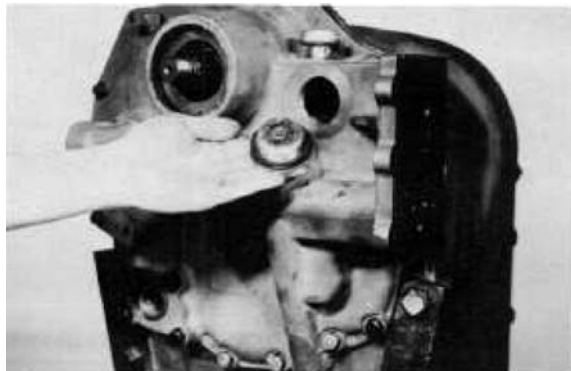
Figure 15 Install front cover plug.
