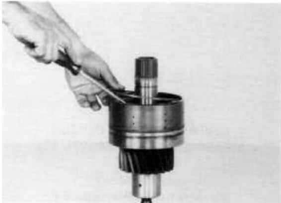
Figure 94 Install end plate retainer ring.
