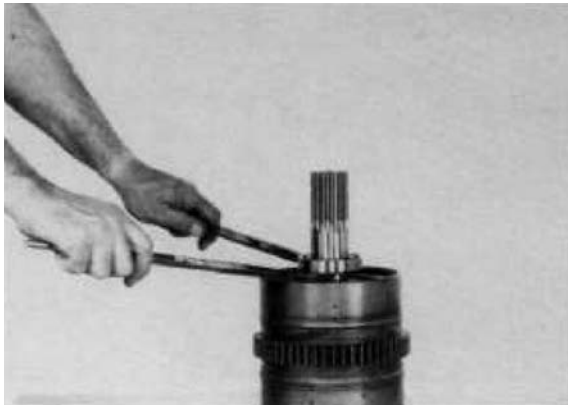
Figure 123 Pry inner bearing up far enough to use a bearing puller.
