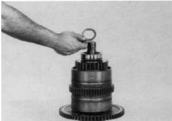
Figure 105 Remove front bearing end plate.
