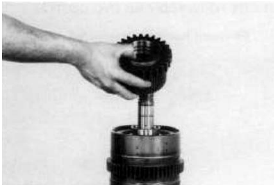
Figure 154 Install clutch gear into clutch drum. Align splines on reverse gear with internal teeth of friction discs. Do not force this operation. Gear splines must be in full position with internal teeth of all friction discs.
