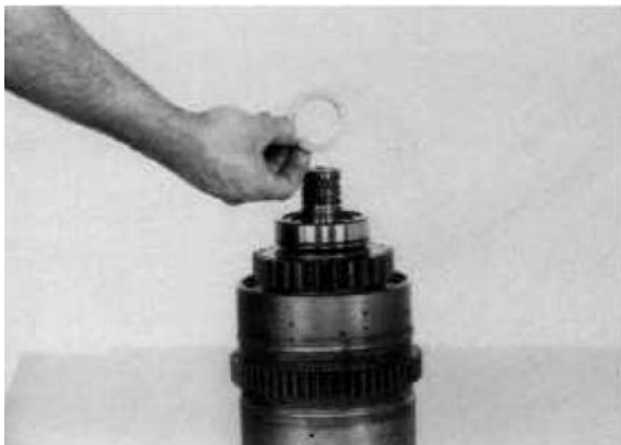
Figure 165 Remove end plate.
