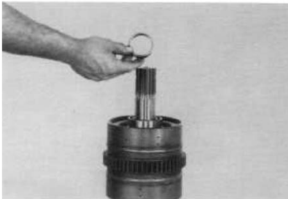
Figure 141 Install clutch gear inner and outer bearing spacer.
