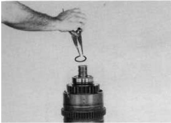
Figure 104 Remove front bearing retainer ring.
