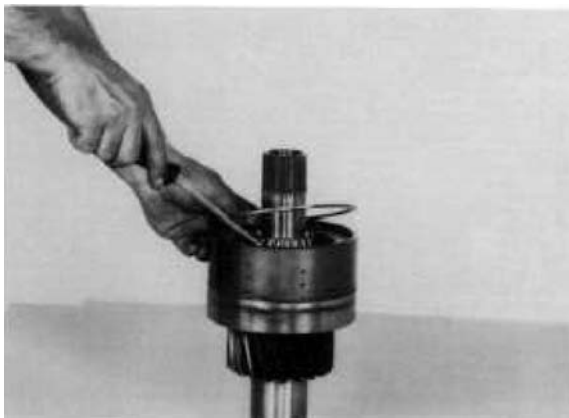
Figure 77 Remove clutch end plate retainer ring.
