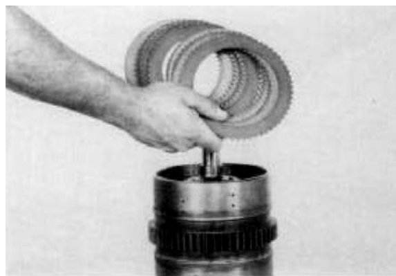
Figure 181 Remove inner and outer clutch discs.
