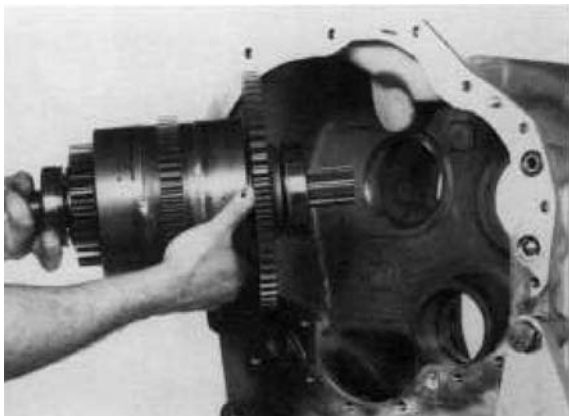
Figure 60 Remove reverse and 3rd clutch assembly.
