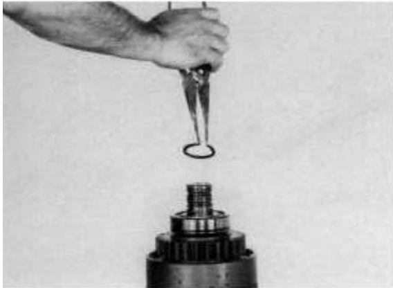
Figure 164 Remove front bearing end plate retainer ring.
