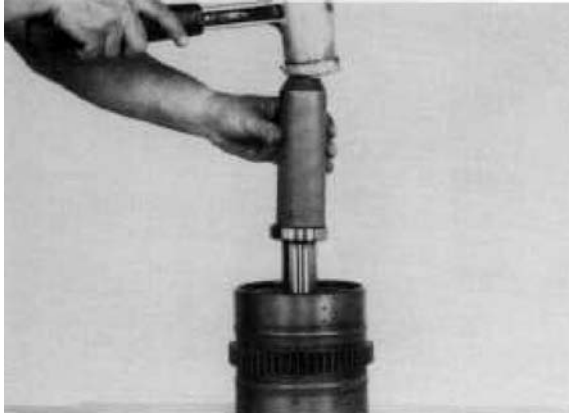
Figure 140 Install clutch gear inner bearing. NOTE: The inner bearing does not have a bearing shield.
