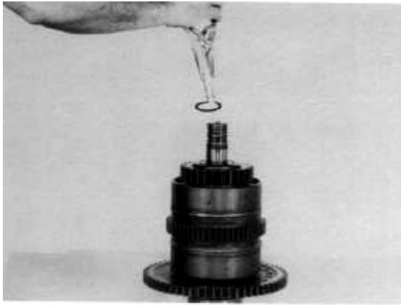
Figure 110 Remove clutch driven gear outer bearing retainer ring.
